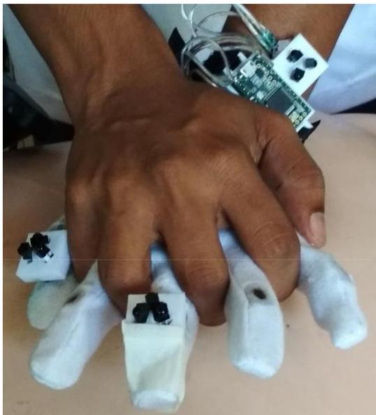
Fig. 6 Glove with three photodiode circuits
