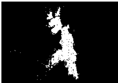
Fig 6: Classification of pixels containing water. Pixels that contain water are shown in white while other pixels are shown in black
